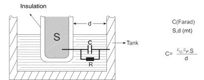
Due to leakage currents and the distance (d) between tank and probe is relatively high, above equation is not practical to use. Therefore, instead of electrical capacity, impedance measurement will provide accurate level results.
