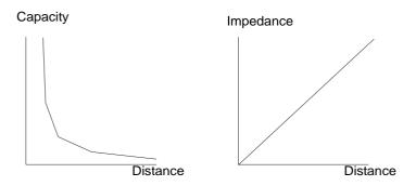
Impedance is  $Z = R + jL\omega + (j\omega)^{-1}$ . R is defined as reel component and represents the medium conductivity.
