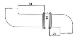
If the closed elbow before and after the check valve, the check valve must be placed at a minimum distance of 5d from the previous elbow and a minimum distance of 2d after the elbow.
