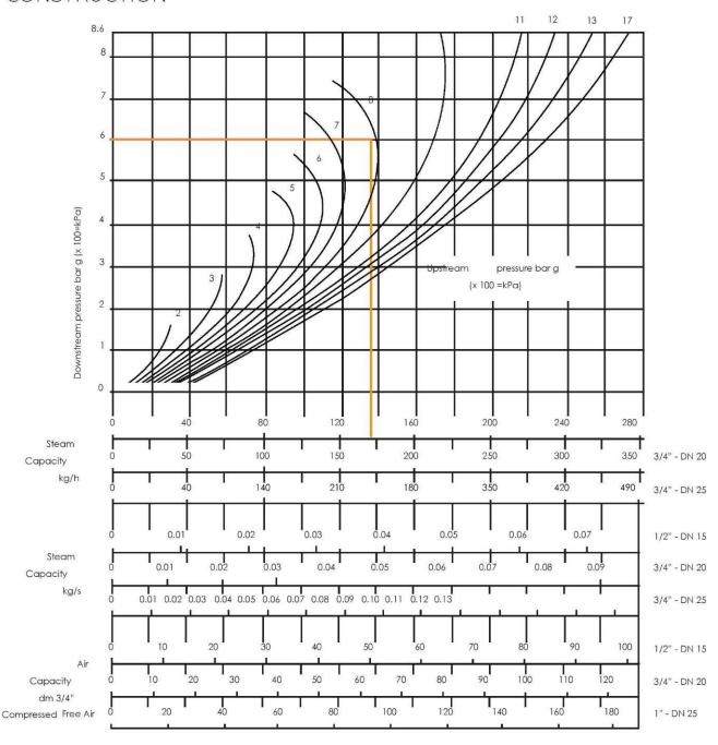
**Example:** required reducing valve to pass 120 kg/h reducing from 8 to 6 bar. From the downstream pressure of 6 bar on the left hand side of the chart to be extended out horizontally until the line. Meets the curve of 8 bar upstream line. Orthographic projection of this point is read as the capacity of the product.
