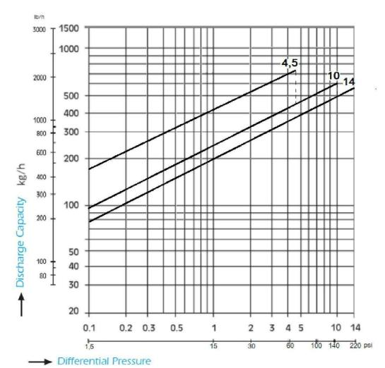
$\Delta P$  = Inlet Pressure / Outlet Pressure
